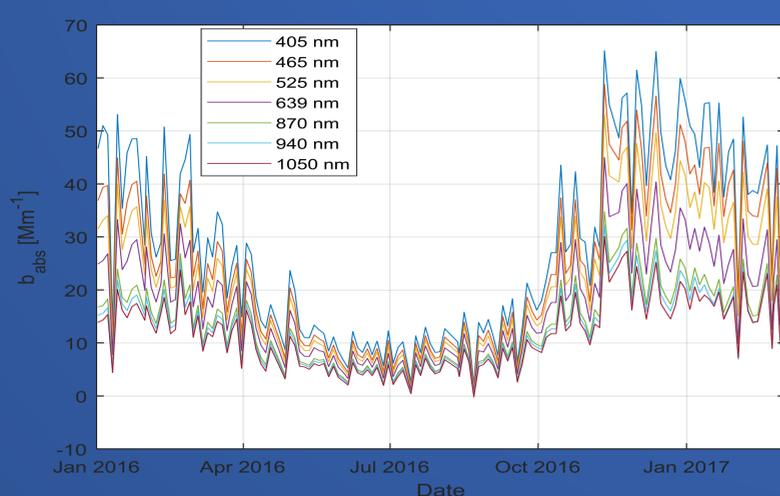
Temporal series of  $b_{abs} [Mm^{-1}]$  for PTFE filters with 0.2 μm pores, for 7 applied wave-lengths by MABI
