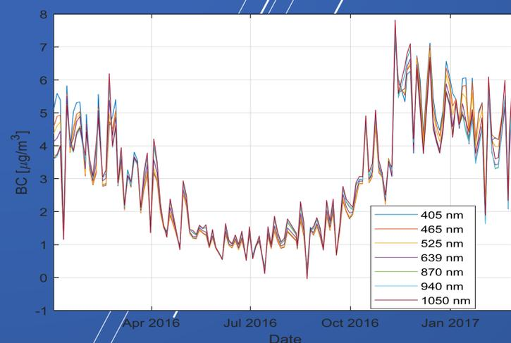
Temporal series of  $BC [\mu g/m^3]$  for PTFE filters with 0.2 μm pores, for 7 applied wave-lengths by MABI
