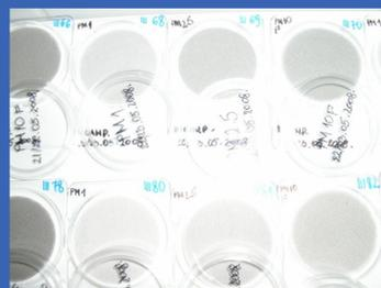
Analysis was done by Multi-wavelength Absorption Black carbon Instrument (MABI) by irradiation of blank and exposed filters with 405nm, 465nm, 525nm, 639nm, 870nm, 940nm and 1050nm light (LEDs).
