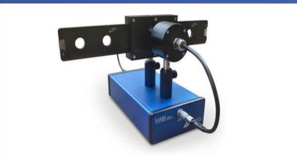
Multi-wavelength Absorption Black carbon Instrument (MABI) developed by ANSTO, Australia
