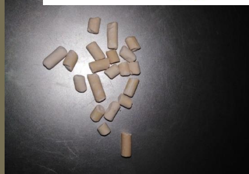
X-type zeolite (Faugazite)
