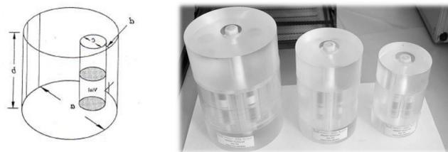
Figure 2: Thyroid phantoms: ANSI (left); SURO (right).
