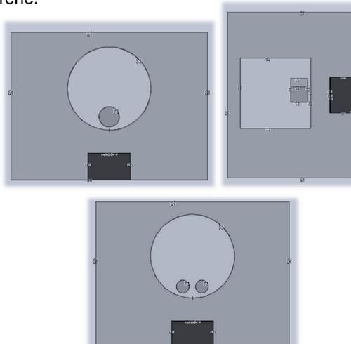
Figure 3: The thyroid geometry and detector model with MC simulation.
